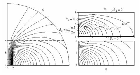
Fig. 2 - Magnetic field pattern: a), c) - calculated wit FEM; b) calculated with (18).
